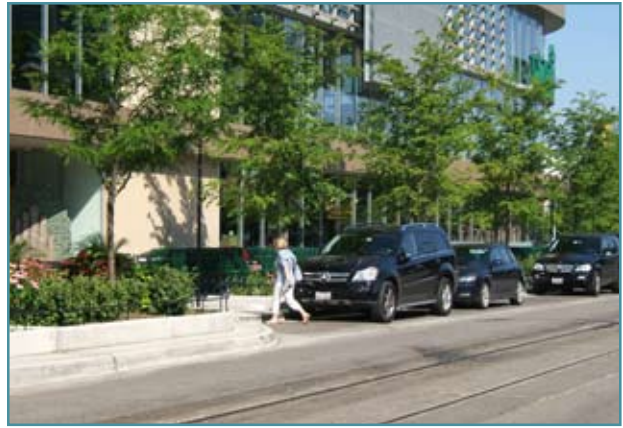
Kingsbury Street at Whole Foods showing landscaped islands to extend curb lines and shadow parking
